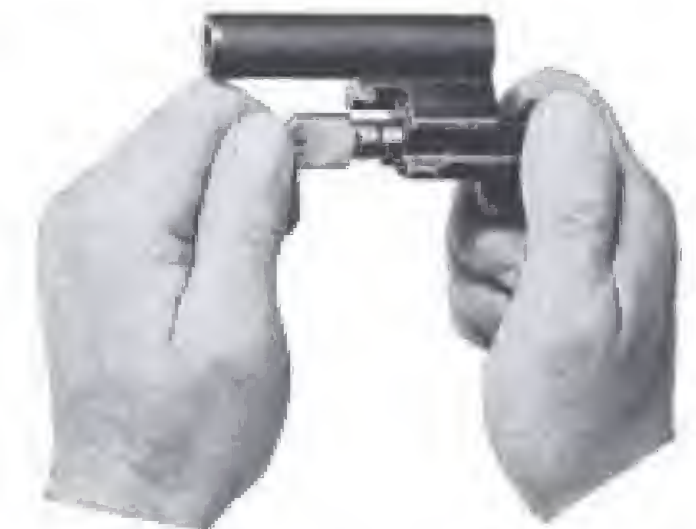
Fig. 34 Stripping the bolt assembly
